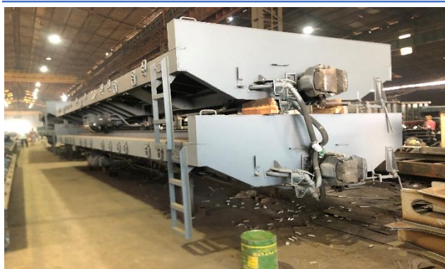
Exhibit 55: Wagon without wheelset and outer structure.
