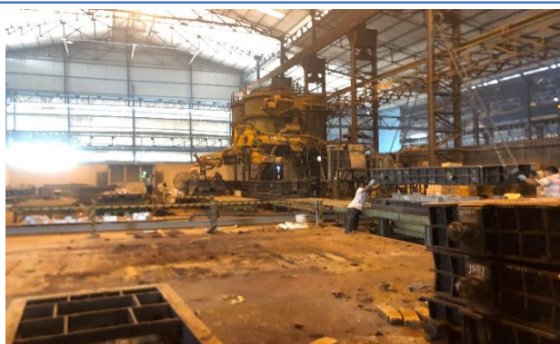
Exhibit 37: Sand Mixture is used to mix sand for molding process.
