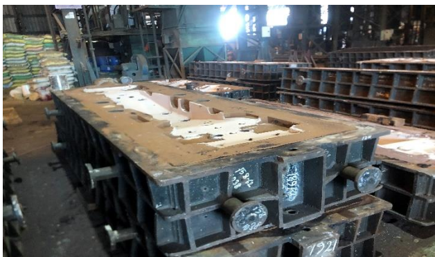
Exhibit 41: Melded Silica Steel poured into mold to make components. The process take around 10 hours.
