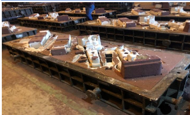
Exhibit 41: Melded Silica Steel poured into mold to make components. The process take around 10 hours.
